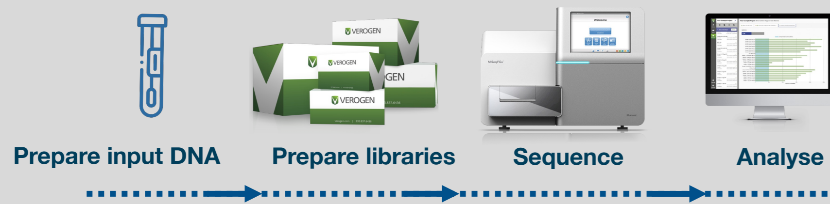
Figure 1. The MiSeq FGx™ workflow. The ForenSeq™ DNA Signature Prep kit is used to prepare libraries for sequencing on the MiSeq FGx sequencer. The analysis of data is automated and integrated into the workflow.
